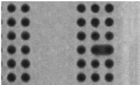
Fault detection also at hidden solder joints
